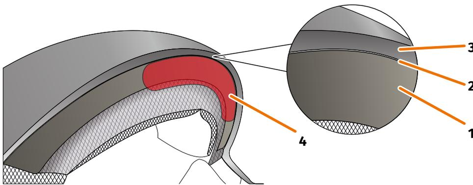
**FIGURE 6 // Gap in helmets without sun visors**
